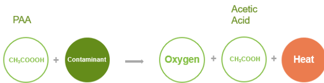
Figure 1: Chemical Decomposition of Peracetic Acid
