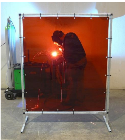
Figure 1: A welder working behind a welding screen.
