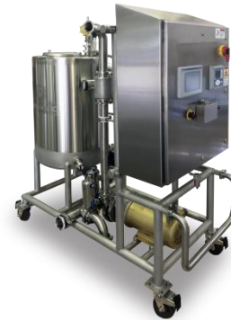
Figure 1: CIP skid example with water tank and control system. Courtesy of Dobbins Company. 2
