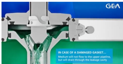
FIGURE 2 : GEA VIDEO EXCERPT - EXAMPLE OF A LEAK AT THE BOTTOM SEAL
